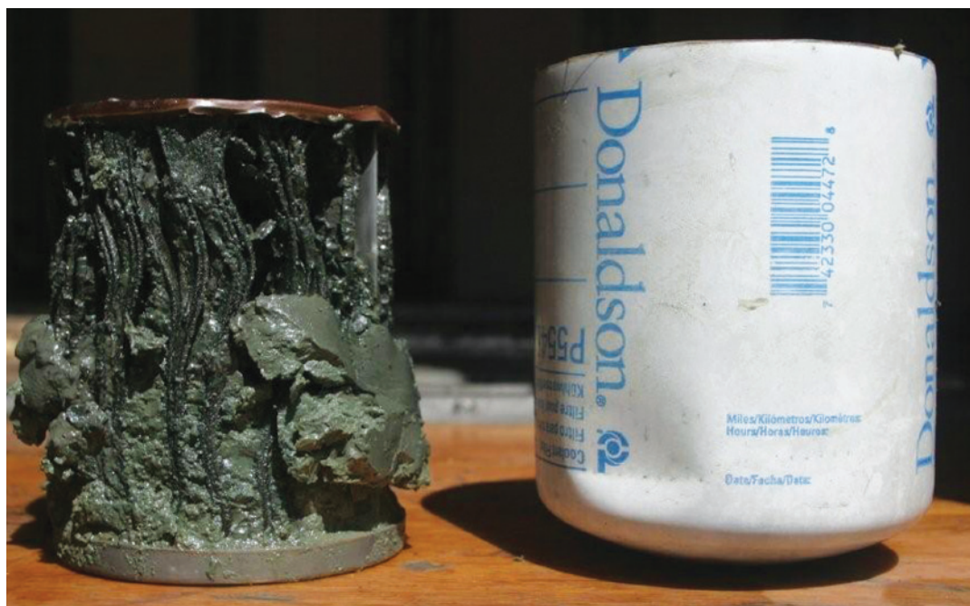
This shows what happens when the additive build up collects in a coolant filter. This is avoided with a waterless coolant. Images courtesy of Evans Cooling Systems.
